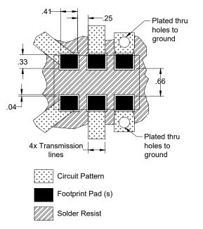
Dimensions are in Millimeters Mounting Footprint
