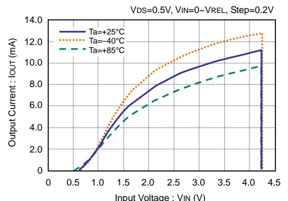
**TYPICAL CHARACTERISTICS – P-ch Driver Output Current vs. Input Voltage**● **VDA2010CTA (CMOS 2.0V)**
