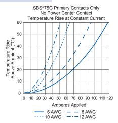
Current - Temperature Derating per IEC 60512-5-2 Test 5B
