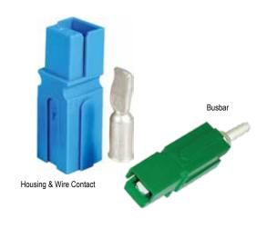
PP180 are the largest of the Powerpole<sup>\*</sup> series housings. They are designed to accommodate up to 3/0 (70 mm<sup>2</sup>) wires and handle high currents up to 350 amps. Busbar contacts are also available for power inputs and takeoffs. Color-coded housings minimize user confusion and the potential of cross mating circuits.
