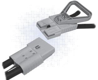
SBE<sup>®</sup> and SBX<sup>®</sup> connectors can integrate up to 8 auxiliary power / signal contacts along with the two primary power circuits. Sequencing within auxiliary positions is possible using the 4 pin lengths available in the 1x4 auxiliary connector. SBE<sup>®</sup> and SBX<sup>®</sup> offer touch safe housings.
