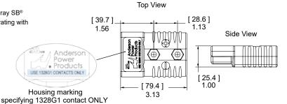
Wires sizes from 10 to 1/0 AWG (5.3 to 50 mm<sup>2</sup>) fit in the second to largest connector in the SB<sup>®</sup> series. The 3 pole SB<sup>°</sup> 175 adds an additional position for power or grounding. All Multipole wire connector housings are genderless and mate to themselves minimizing inventory and assembly complexity.
