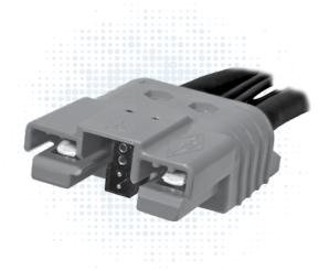
SBE<sup>®</sup> and SBO<sup>®</sup> connectors build on the capability of the two pole SB<sup>®</sup> connectors by offering up to 8 auxiliary power / signal contacts along with an IEC 60950 touch safe housing. The center of the main connector features a connector holder for either: two PP15-45, two PPMX, or APP's innovative 1x4 auxiliary connector.
