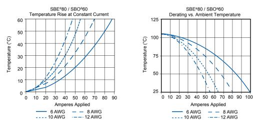
NOTE: Temperature rise charts are based on a 25°C ambient temperature.
