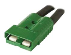
The SB<sup>\*</sup> 350 is the largest connector in the series with power capabilities up to 500 amps with a 350 mcm wire. Wires ranging from 1/0 to 350 mcm (53.5 to 185 mm<sup>2</sup>) fit into the one piece housing available in standard PC or a chemical resistant PBT/PC blend. Silver plated wire or busbar contacts minimize electrical resistance while offering supreme durability and reliability.
