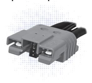
SBE® and SBO® connectors build on the capability of the two pole SB® connectors by offering up to 8 auxiliary power / signal contacts along with an IEC 60950 touch safe housing. The center of the main connector features a connector holder for either: two PP15-45, two PPMX, or APP's innovative 1x4 auxiliary connector.
