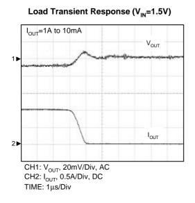
Load Transient Response (V<sub>IN</sub>=1.5V)
