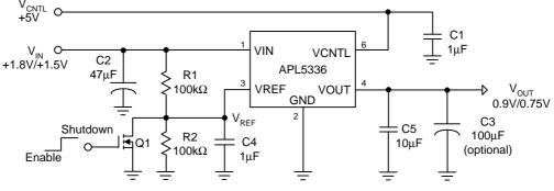
The ceramic capacitor C5 ( at least 8µF) is necessary for output stability.
