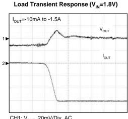
CH1: V<sub>OUT</sub>, 20mV/Div, AC CH2: I<sub>OUT</sub>, 0.5A/Div, DC TIME: 1µs/Div
