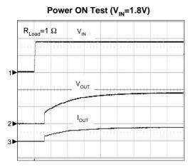
CH1: V<sub>IN</sub>, 1V/Div, DC CH2: V<sub>OUT</sub>, 500mV/Div, DC CH3: I<sub>OUT</sub>, 1A/Div, DC TIME: 50ms/Div
