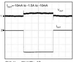
CH1:  $V_{OUT}$ , 20mV/Div, AC CH2:  $I_{OUT}$ , 0.5A/Div, DC TIME: 200 $\mu$ s/Div
