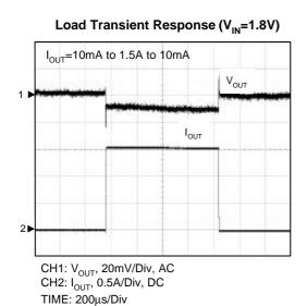
Load Transient Response (V<sub>IN</sub>=1.8V)
