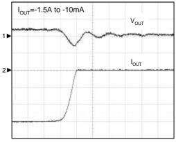
$<sup>\</sup>begin{array}{c} \text{CH1: } \text{V}_{\text{OUT}}, \text{ 20mV/Div, } \overrightarrow{\text{AC}} \\ \text{CH2: } \text{I}_{\text{OUT}}, \text{ 0.5A/Div, } \text{DC} \\ \text{TIME: } 1 \mu \text{s/Div} \end{array}$
