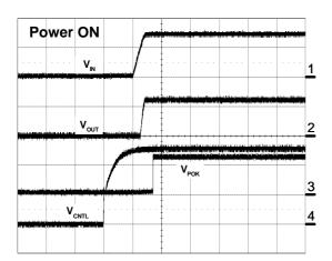
$\begin{array}{l} Ch1: V_{\text{IN}}, 1V/div\\ Ch2: V_{\text{OUT}}, 1V/div\\ Ch3: V_{\text{POK}}, 1V/div\\ Ch4: V_{\text{CNTL}}, 2V/div\\ Time: 10ms/div \end{array}$
