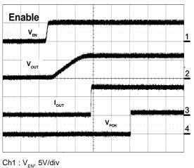
$\begin{array}{l} \text{Ch1}: \ V_{\text{EN}}, \ \text{SV/div}\\ \text{Ch2}: \ V_{\text{OUT}}, \ 1\text{V/div}\\ \text{Ch3}: \ I_{\text{OUT}}, \ 1\text{A/div}\\ \text{Ch4}: \ V_{\text{POK}}, \ 1\text{V/div}\\ \text{Time}: \ 1\text{ms/div}\\ \end{array}$
