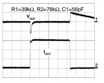
$\begin{array}{l} Ch1 \ : \ V_{_{OUT}}, \ 100mV/Div\\ Ch2 \ : \ I_{_{OUT}}, \ 500mA/Div\\ Time : \ 20\mu s/Div \end{array}$
