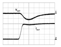
$\begin{array}{l} Ch1 \hspace{0.2cm} : \hspace{0.2cm} V_{\text{OUT}}, \hspace{0.2cm} 100mV/Div \\ Ch2 \hspace{0.2cm} : \hspace{0.2cm} I_{\text{OUT}}, \hspace{0.2cm} 500mA/Div \\ Time : \hspace{0.2cm} 1\mu s/Div \end{array}$
