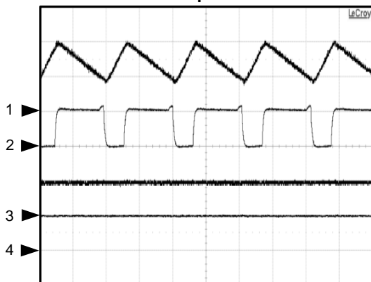
Boost Mode, V_{BAT}=3.8V , I_{VBUS}= 500mA , In CCM Operation
