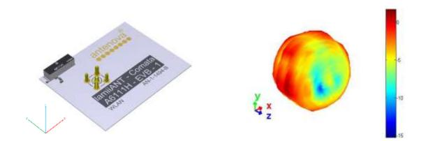
**3D pattern at 2450 MHz** Drag to rotate pattern and PCB by using Adobe Reader (Click to Activate)
