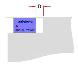
Additional ground and components near the antenna should be at a distance of at least 2 mm. Where possible the antenna should be clear of ground from both sides, although the antenna can work well with a minimum clearance of  $D \ge 2$  mm as shown in the drawing above.
