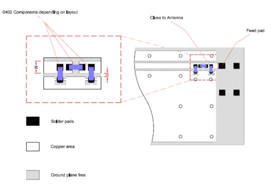
The antenna feed pad is indicated in the drawing above. Additional pads are for mechanical attachment only and should not be grounded.
