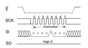
During an Recall operation, all commands will be ignored except the RDSR instruction. In case no command will be sent after RECALL cycle completion a new RECALL cycle will be initiated with the rising edge of  $\overline{E}$ .
