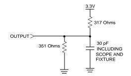
Figure 1. AC Output Loading
