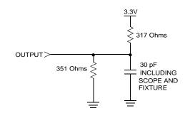
Figure 1. AC Output Loading
