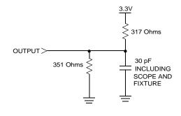
Figure 1. AC Output Loading
