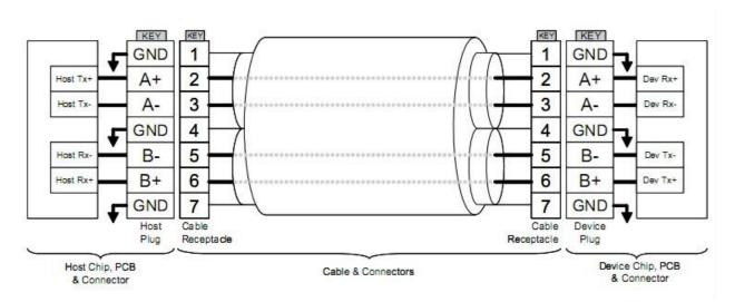
Figure 1-2 SATA Cable/Connector Connection Diagram
