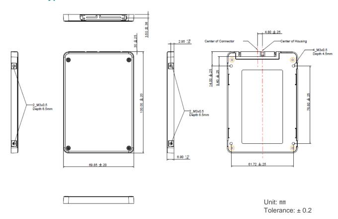
Figure 6-1 7mm Housing Physical Dimensions
