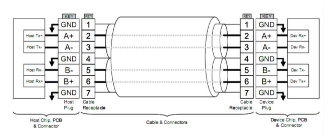
Figure 1-2 SATA Cable/Connector Connection Diagram
