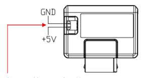
For external power cable connection: this feature is available as an option for Standard Type.
