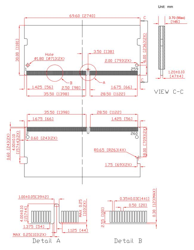
(All dimensions are in millimeters with ±0.15mm t lerance unless specified otherwise.)
