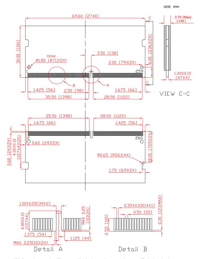
(All dimensions are in millimeters with  $\pm 0.15$ mm t lerance unless specified otherwise.)
