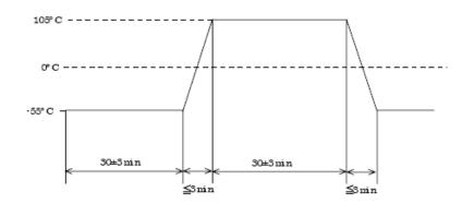
Fig. 6 Rapid temperature change profile
