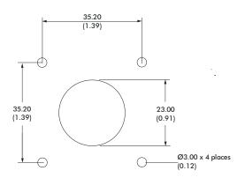
The body of the joystick is mounted from beneath the panel. The boot is passed through the panel cut-out and is held onto the front face of the panel by the mounting bezel. The square bezel has a gloss finish and is designed for use with No.4 x 3/8" pan head self tapping screws whereas the circular bezel has a matt finish and is designed for countersunk screws.
