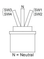
Two switches will actuate as the joystick moves away from center, in either direction.
