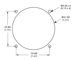
The joystick is dropped into the panel cut-out. The joystick and boot must be kept in place by bezel (option 6 & 7). For panel thickness of <3mm, M3 x 16 countersunk machine screws are recommended.
