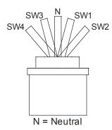
One switch will actuate after 50% of travel, with a further switch at the end of travel, in either direction.
