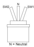
One switch will actuate as the joystick moves away from center in either direction.
