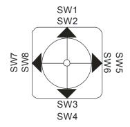
Two switches will actuate in each of the four directions: North, South, East & West.
