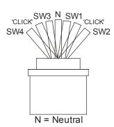
As per option D, but with a mechanical detent between actuation of the first and second switch.
