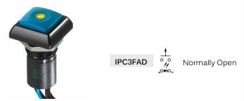
For THIN flying leads, replace F with W. Wire colors: black: NO contact, red: LED anode(+), blue: LED cathode(-) Shown with standard flying lead terminals.
