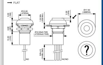
Pushbutton switches for harsh environments • bushing Ø 12 mm • momentary
