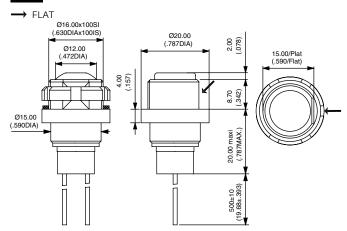
Rear mounted sealed pushbutton switches • bushing Ø 16 mm • latching
