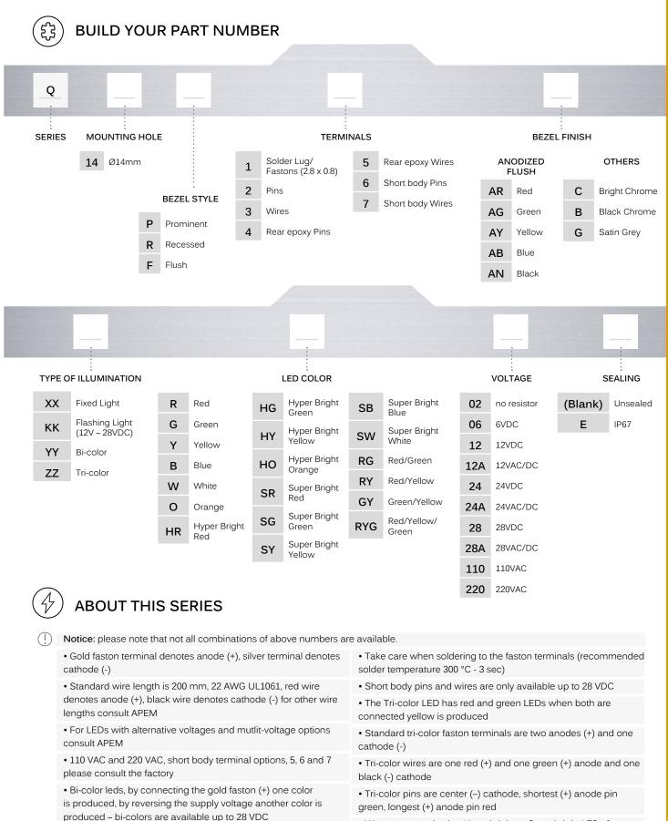
$\bullet$  We recommend using Hyperbright or Superbright LEDs for use at 110 VAC and 220 VAC
