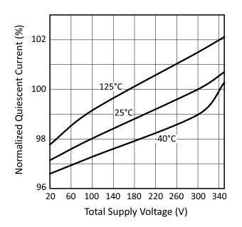
**Figure 14: Power Supply Rejection**
