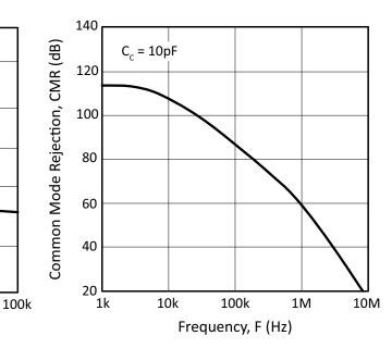
Figure 13: Common Mode Rejection
