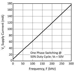
Figure 6: V<sub>DD</sub> Supply Current
