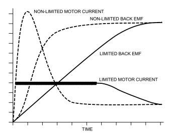
**Figure 17: Current Limit Waveforms**
