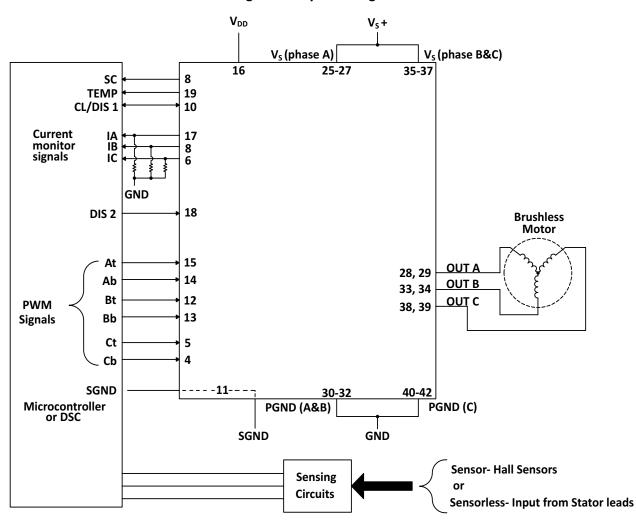
Figure 13: System Diagram
