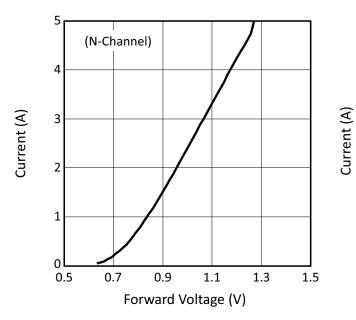
Figure 12: Diode Forward Voltage - Top FET
