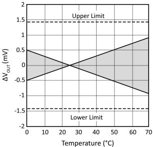
Figure 5: V<sub>OUT</sub> vs. Temperature (VRE410LS)
