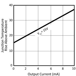
Figure 7: Junction Temp Rise vs. Output Current
