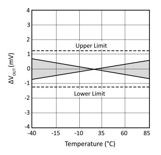
Figure 3: V<sub>OUT</sub>vs. Temperature (VRE410BS)
