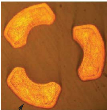
Au/Ni Barrier (Uniform plating thickness)
