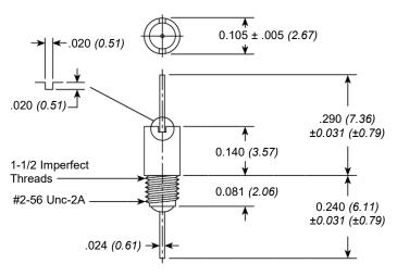
Built and tested in accordance with MIL-PRF-15733. Dimensions in inches (mm)
