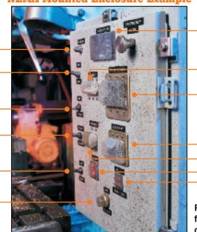
Lever style back-of-panel mounted circuit breaker boots
