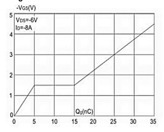
**Figure 5: Gate Charge Characteristics**
