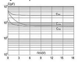
**Figure 6: Capacitance Characteristics**
