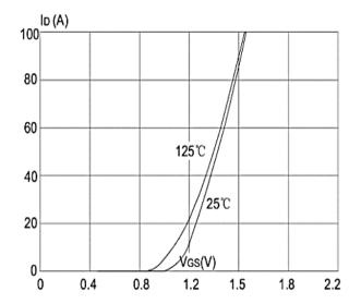
**Figure 2: Typical Transfer Characteristics**
