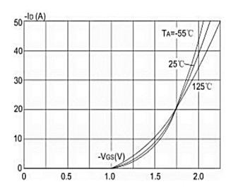
**Figure 2: Typical Transfer Characteristics**
