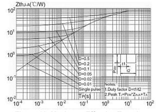
Figure.11: Maximum Effective Transient Thermal Impedance, Junction-to-Case
