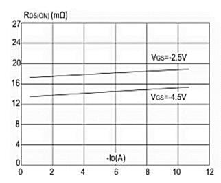
Figure 3:On-resistance vs. Drain Current
