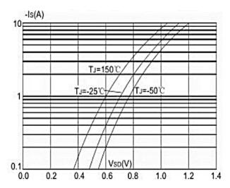
**Figure 4: Body Diode Characteristics**
