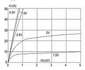
Figure1: Output Characteristics
