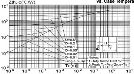
Figure.11: Maximum Effective Transient Thermal Impedance, Junction-to-Case
