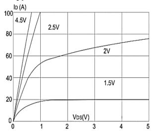
Figure1: Output Characteristics
