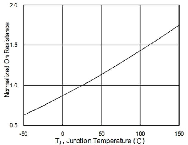
**Fig.6 Normalized R<sub>DS(on)</sub> v.s T<sub>J</sub>**
