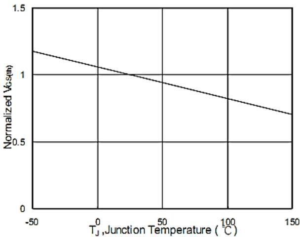
**Fig.5 Normalized V<sub>GS(th)</sub> v.s T<sub>J</sub>**
