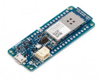
Arduino MKR1000 has been designed to offer a practical and cost effective solution for makers seeking to add Wi-Fi connectivity to their projects with minimal previous experience in networking. It is based on the Atmel ATSAMW25 SoC (System on Chip), that is part of the SmartConnect family of Atmel Wireless devices, specifically designed for IoT projects and devices.
