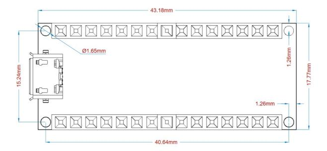
Mechanical dimensions of Arduino Nano RP2040 Connect
