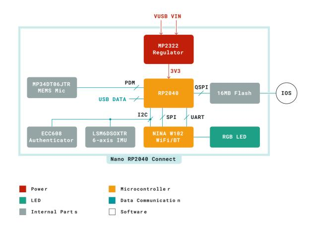
Block Diagram of Arduino Nano RP2040 Connect
