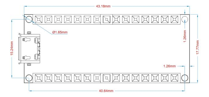
Mechanical dimensions of Arduino Nano RP2040 Connect
