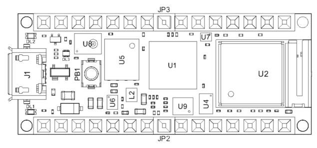
Front View of Arduino Nano RP2040 Connect Topology
