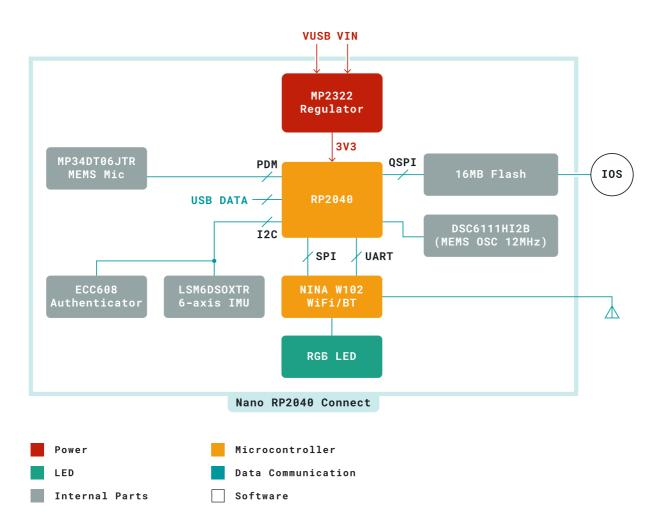
Block Diagram of Arduino Nano RP2040 Connect
