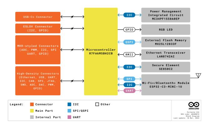
Figure 3. High-level architecture of the Portenta C33
