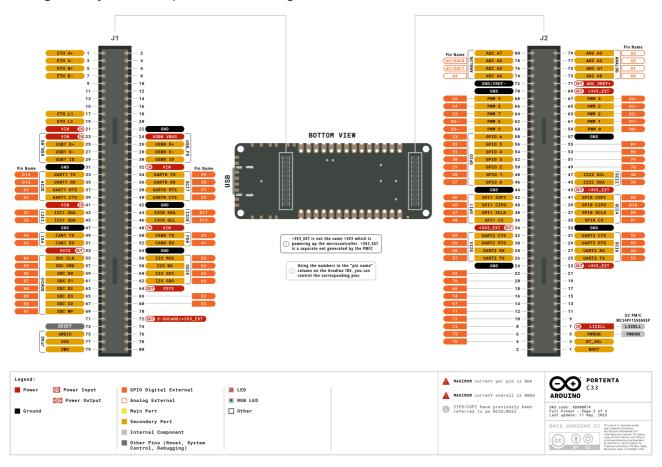
Figure 2. Portenta C33 pinout (High-Density connectors)
