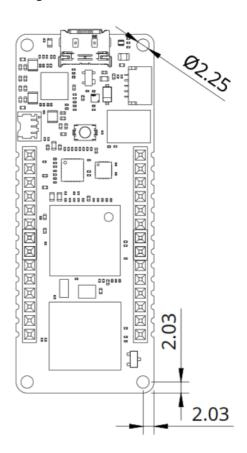
Figure 5. Portenta C33 board outline (left) and mounting holes dimensions (right)
