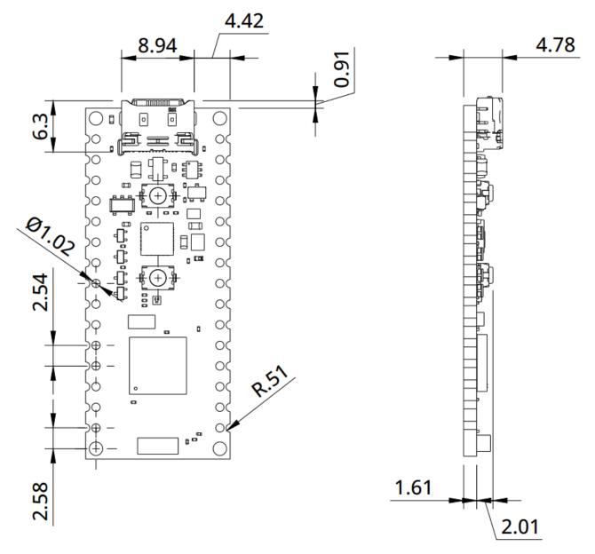
The Nano Matter was designed to be usable as a surface-mount module and presents a dual inline package (DIP) format with the Nano-styled header connectors on a 2.54 mm pitch grid with 1 mm holes.
