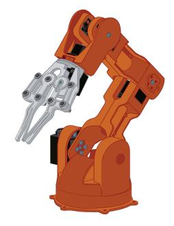
You can assemble your **BRACCIO** in a multitude of ways. Because it is designed for versatility, the BRACCIO can also support various objects on the end of the arm. The included BRACCIO shield allows you to hook up the servos directly to your Arduino board.
