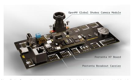
Example of a typical installation for a solution including Portenta H7 and Global Shutter Camera Module. A Portenta board must be connected for operation of the Portenta Breakout Board.
