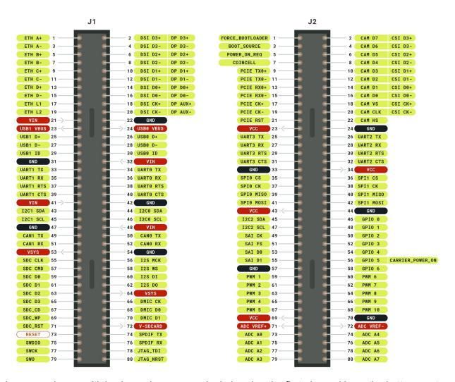
In cases where multiple channels are on a single header, the first channel is on the bottom part of the header and the section channel is on the top part of the header. The order of the channel is determined by the silkscreen markings.
