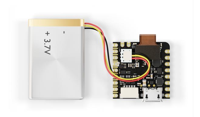
Example of a typical solution for remote machine vision including an Arduino® Nicla Vision and battery. Notice the orientation of the battery's cable in the board's connector.
