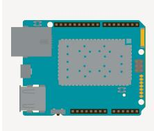
**ARDUINO YÚN REV 2** is an improved version of the well known Linux based system board that enables advanced network connections. You can connect it either to a wireless or wired network.
