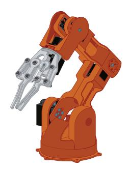
You can assemble your **BRACCIO** in a multitude of ways. Because it is designed for versatility, the BRACCIO can also support various objects on the end of the arm. The included BRACCIO shield allows you to hook up the servos directly to your Arduino board.
