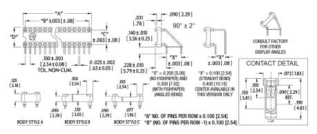
ALL DIMENSIONS: INCHES [MILLIMETERS] ALL TOLERANCES: ±0.005 [0.13] UNLESS OTHERWISE SPECIFIED FOR VERTICAL MOUNTING, SEE DATA SHEET 13002 **CONSULT FACTORY FOR OTHER SIZES AND CONFIGURATIONS**
