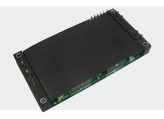
Advanced Energy's Artesyn AGF700 series isolated DC-DC converter is designed for the type of RF power amplifiers used in micro and macro cell, NodeB/eNodeB and remote radio head (RRH) telecommunications applications.
