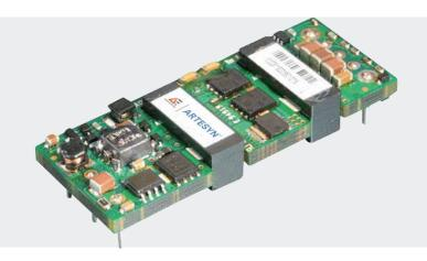
Advanced Energy's Artesyn AVO75 series of eighth-brick isolated DC-DC converters comprises six single output models offering fully regulated voltages of 1.2 V, 1.8 V, 2.5 V, 3.3 V, 5.0 V or 12.0 V. These converters can deliver up to 25 amps and up to 75 watts of output power, depending on the particular model. They have a wide 2:1 input range of 36 to 75 Vdc and are designed primarily for use with standard 48 V telecommunications equipment supplies.
